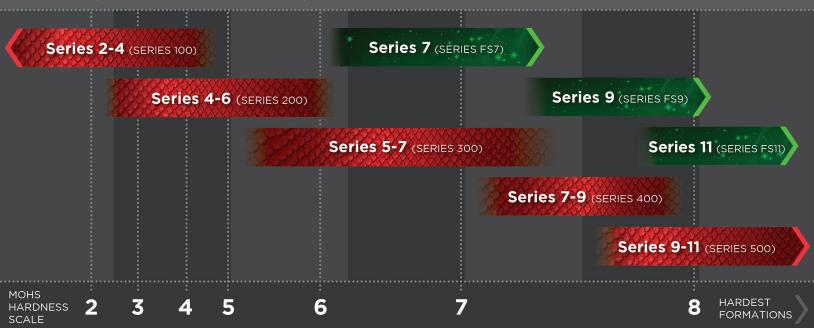
If the crown tends to polish or cut too slowly with the available bit weight, the formation may not be abrasive enough to expose new diamonds: try using the next higher SERIES bit which will allow the matrix to wear easier. Switching to a turbo waterway may also help prevent polishing; it has less surface area and the restricted flow promotes regrinding of the cuttings to stripping away the matrix.
